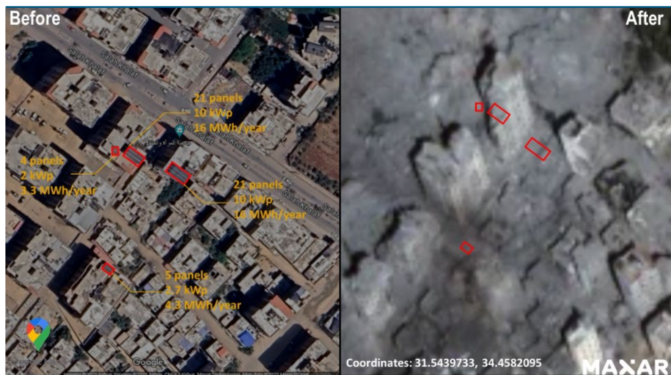
Figure 1. Satellite images of PV systems before and after being destroyed near Al Shati refugee camp in northern Gaza
